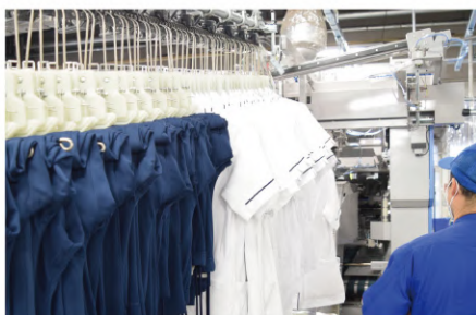
● Jackets and pants are fed without sorting works.
