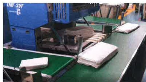
▲ Collective transfer by conveyer system
