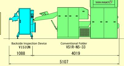
New VS1V-N5-33 + VISION (Backside Inspection
