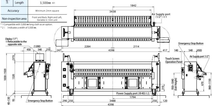
\$1 The height of Air Supply port from the floor varies according to the machine height adjustment. \$2 1 The height of Power Supply port from the floor varies according to the machine height adjustment. \$3 The drawing above shows the dimensions of 3,300mm width machine.
