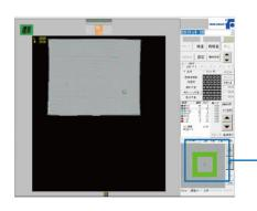
If any defect is found during inspection, the defect area is marked by color and displayed. The area can be displayed with up to 16 times expansion.
