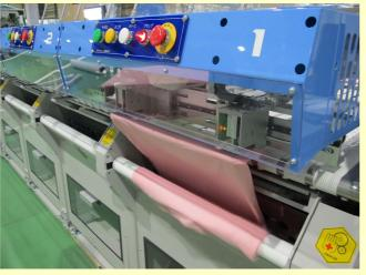
With conventional feeders, straightening wrinkles often hindered productivity. With our new feeder, after putting pillowcases into clamps, counting on the machine, you can immediately start preparation for the next pillowcase.
