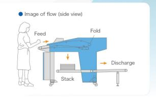
Applicable linen: Face towel, Wash towel, Cleaning cloth, etc Feedable size: 2 half fold: W430 x L 1000mm 1 half fold: W 430 x L850mm
