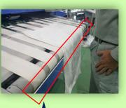
Feeding Guide equipped to make it easier to find the center of placing positions and the tips.
